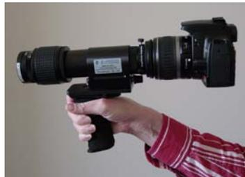
Note: Since the camera is now on “manual focus”, the focus ring on the eyepiece might need to be adjusted for best possible focus. Also, once the camera is attached to the CoronaFinder, the lens manual focus ring can be rotated slightly to change focus.
