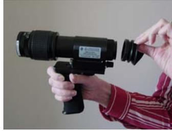
2. ScopeTronix AdaptaView should be attached to front of camera.
