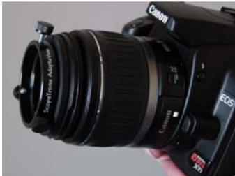
3. Make sure camera lens is set to manual focus (MF).
