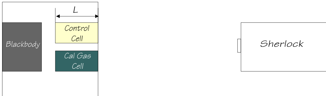
Figure 8. Standard setup for concentration calibration of the Sherlock camera using standard gas cells.
